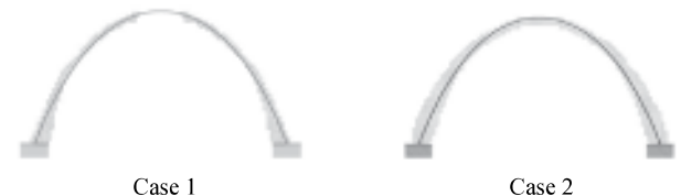
Fig.5 Cross sections of results and corresponding catenaries
